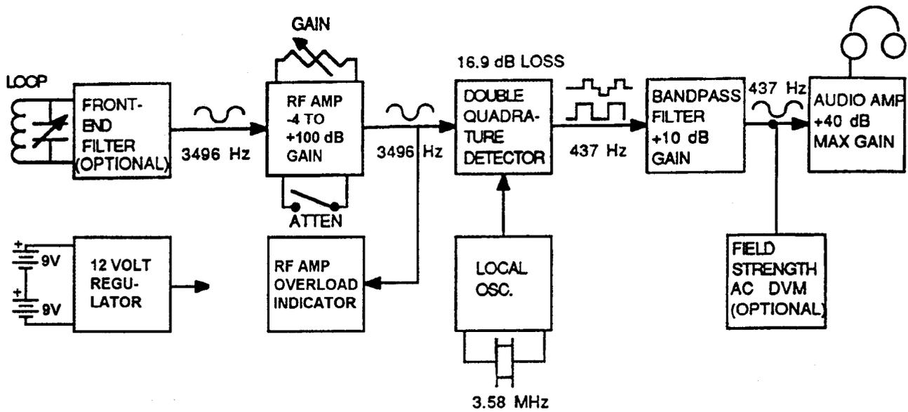
DOUBLE-QUADRATURE DETECTOR AND LOCAL OSCILLATOR USED IN ABOVE RECEIVER
