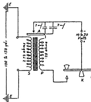
Like near-field magnetic induction, earth-dipole propagation has an inherent range limitation in that signal strength varies inversely as the cube of the distance from the source (in a uniformly-conductive earth). The relevant equation (from [5]) is:
