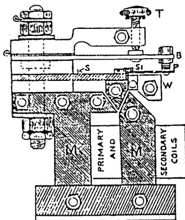
Drawing and circuit of the French "Parleur" power buzzer, model "2 ter". Initially, British power buzzers were made to this design.
