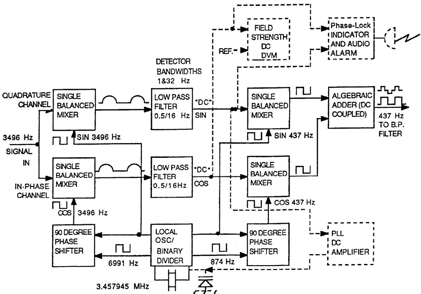
Figure 2a Beacon Receiver Schematics
