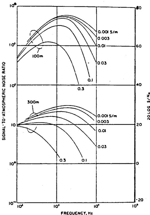
**Figure 1.** Ratio of magnetic field strength to atmospheric noise on the surface directly over a transmitting loop with magnetic moment of 1000 (amp-turns-sq metres). Receiver bandwidth is 10 Hz. Path lengths of 100 m and 300 m are shown, with ground conductivity of 0.001 - 0.3 mho/m.
