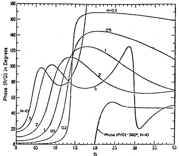
**Figure 3.** The difference in phase between the horizontal and vertical magnetic fields on the surface over a buried loop antenna.
