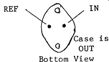
Figure 2. LM 317K Connections
