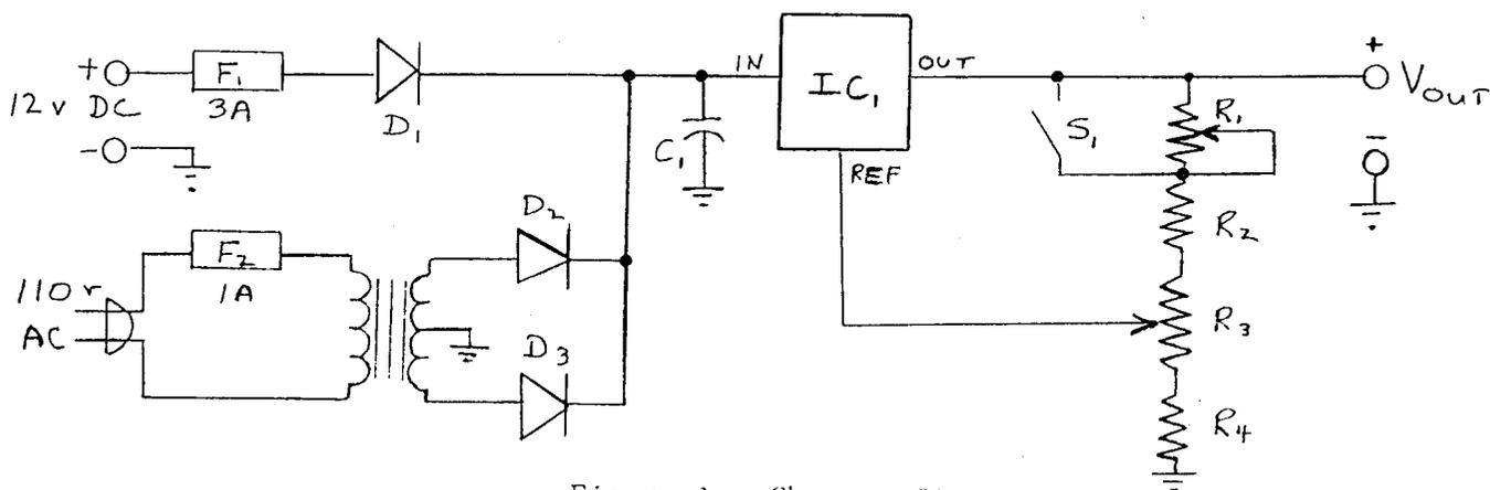
Figure 1. Charger Circuit
